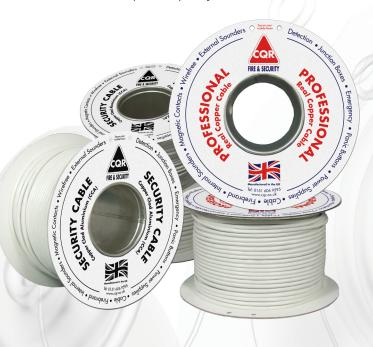
This UK manufactured cable has cores of 7 strands of 0.182mm annealed tinned copper wire and is sheathed in Type 1 PVC. Suitable for any installation where signal integrity is paramount.
